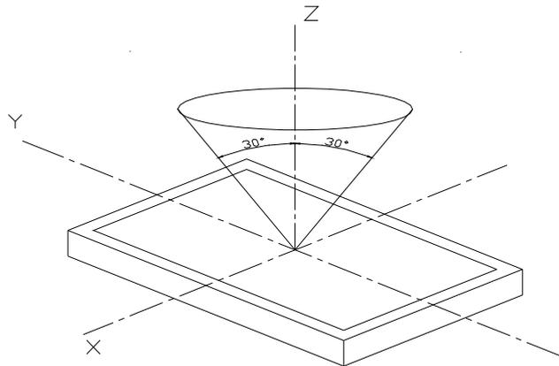
*Inspection should be performed within angle  $\phi$  ( $\phi$  is usually  $30^\circ$ ) from Z axis to each X and Y.*
